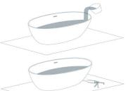
Before final fixing check that the bath is level and connected to the plumbing system, by adding water and ensuring it drains away adequately leaving no puddles and that there are no leaks. Once checked, half fill the bath to ballast it before securing it to the floor. Apply silicone adhesive evenly between the base of the bath and the floor filling the 1-2mm gap.
