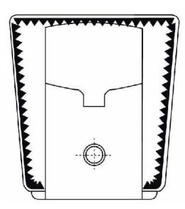
To optimize the fixing at wall of sanitaryware, apply the self-sticking seal on its back as shown in the picture.
