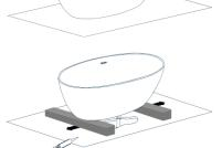
In most instances the waste will have to be recessed into the floor and connected using a flexible fitting. Once the pipe work is completed and ready to receive the bath we recommend raising the bath on a number of
