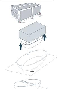
Carefully remove the box from the wooden crate ensure you are extra careful when dismantling the wooden crate. Lift the box carefully over the top of the bath.
