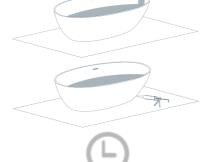
To ensure the best result leave the water in the bath 10-12 hours or overnight while the silicone adhesive sets.
