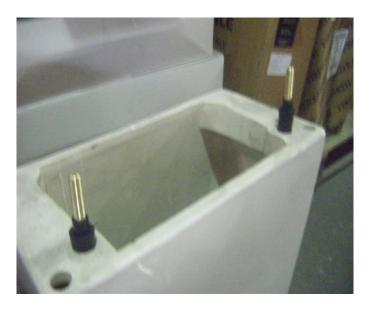
• Thread a nut on to the brass thread, slide the expanding rubber bushes on to the brass thread, place a washer and nut on to the brass thread and tighten to slightly expand the rubber bushes (E)
