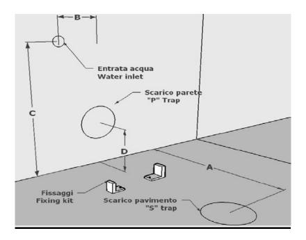
Position the water connection in the wall – 220mm from the floor and 90mm to the left of the soil pipe centre according to the table below
