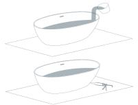
Before final fixing check that the bath is level and connected to the plumbing system, by adding water
